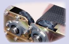
Heavy duty belts with self cleaning head and tail pulleys. Easy access grease ports. Fixed exit length.
